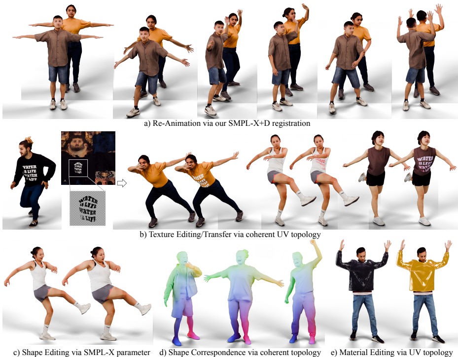
Fig. 1: Applications enabled by AvaImg. Because all registrations share SMPL(-X) parameter space and a coherent UV layout, our output directly supports re-animation, texture editing and transfer, shape editing, dense correspondence, and material editing.
