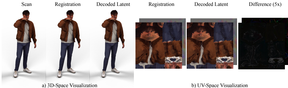
Fig. 5: VAE roundtrip validation. (a) Original scan, AvaImg registration, and mesh from VAE-decoded UV maps are visually near-indistinguishable. (b) Original UV maps, VAE-reconstructed, and 5\times amplified difference.
