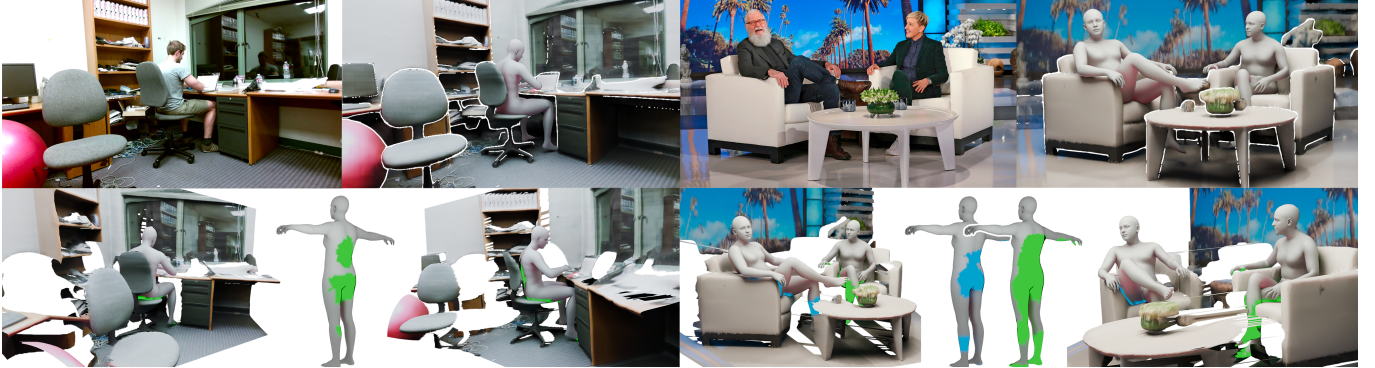
Fig. 1. Given a single monocular RGB image containing a human in a complex environment, PhySIC reconstructs metrically aligned 3D human and scene geometries as well as a dense vertex-level contact map. Our method jointly optimizes human pose, scene geometry, and global scale to produce a physically plausible human-scene pair, accurately capturing contact and interactions such as sitting and foot-floor adherence, even in the presence of occlusions. Image.
